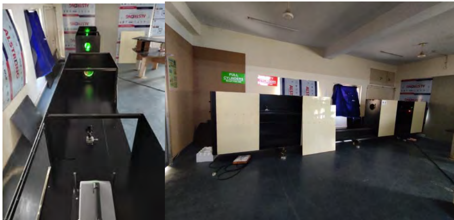
Photographs of the developed high-speed Schlieren imaging system
