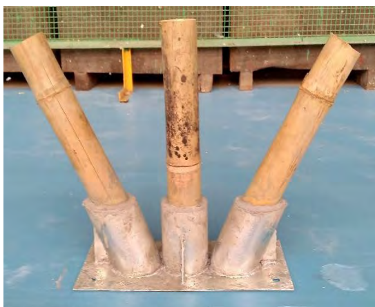
Fig.: Bamboo joints (sample) and joints under mechanical testing
