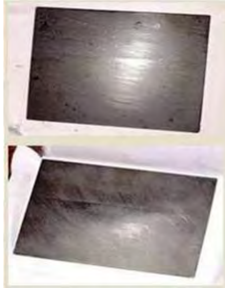
Tiles developed from industrial waste for anechoic chamber fabrication
