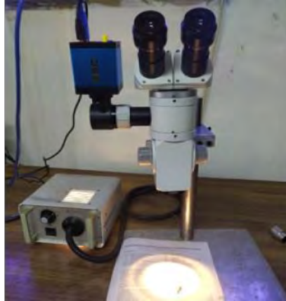
Integration of optical head prototype with camera module
