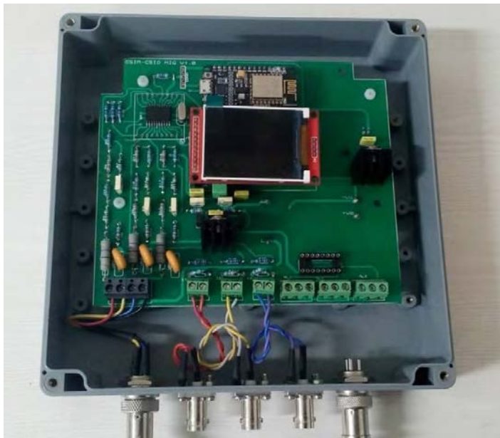
View of the developed Wi-Fi enabled Wireless Power Meter
