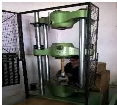
Fig.: Bamboo joints (sample) and joints under mechanical testing
