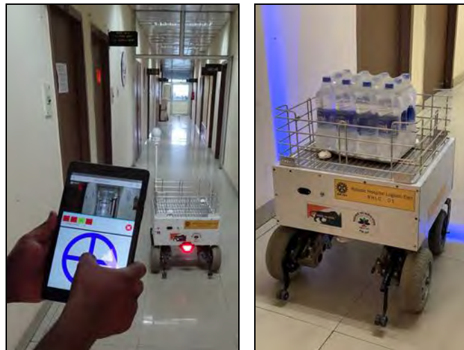
Android Tablet based wireless control for Robotic Hospital Logistic Cart
