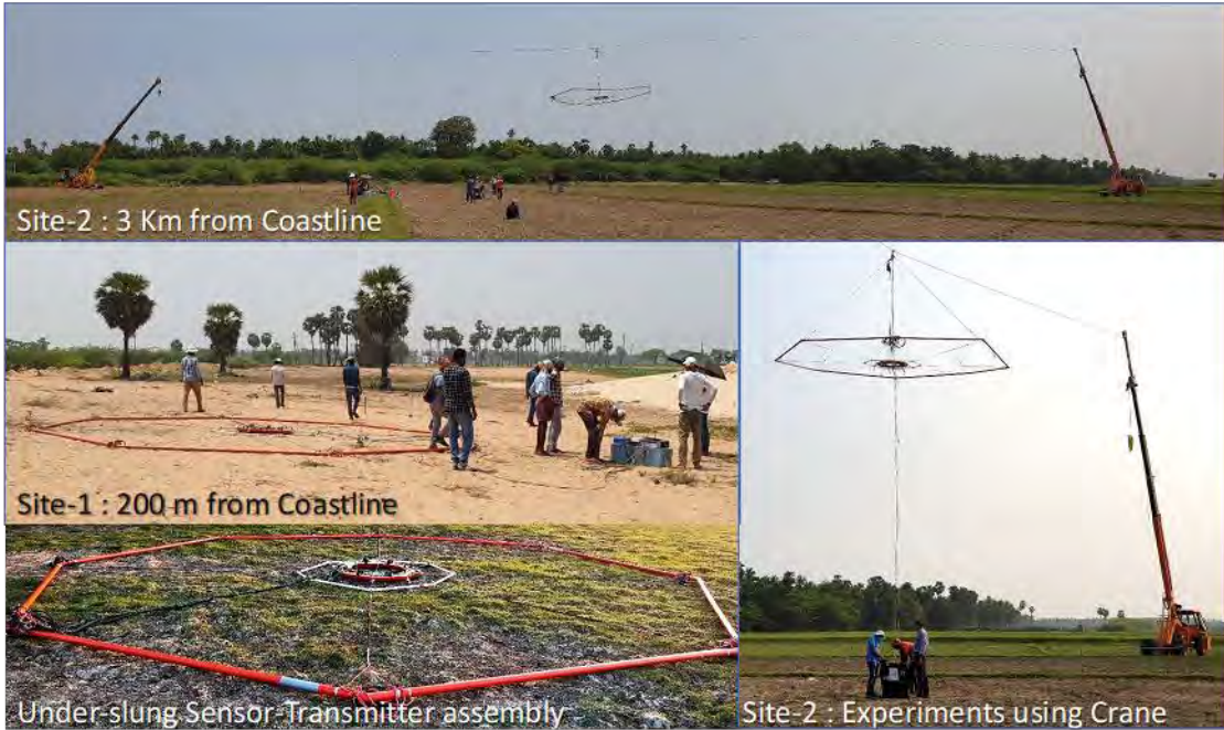
Target Detection Experiment with the integrated DREAM system at Coastal Site (Ongole, AP, India) during March 2021
