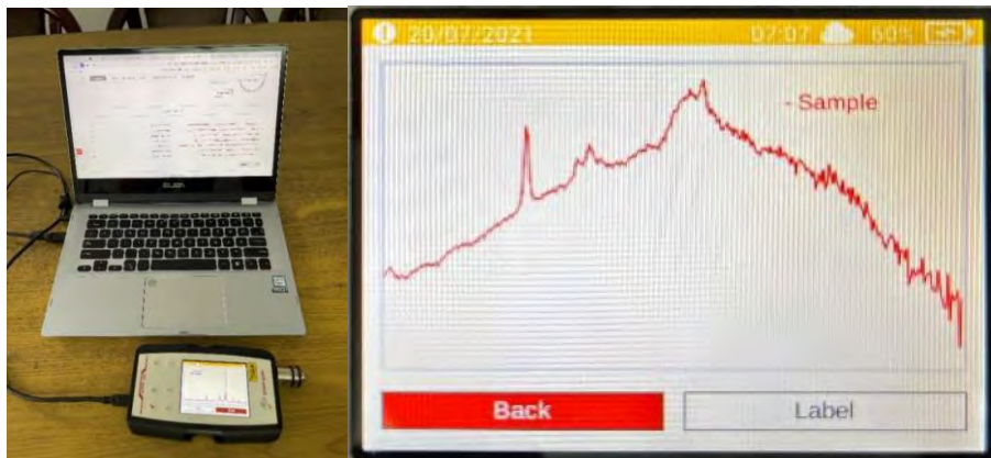
Experimental set-up for narcotics detection system and the Raman Signature
