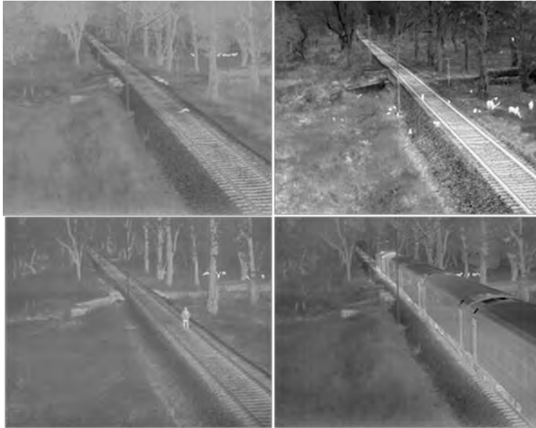
Thermal images of some of the objects captured by eleThermAlert in different environment conditions (Left-Right, Top-Bottom - Midnight: Mongoose & Deer, Afternoon: Monkey & Deer, Sunrise: Human & Deer, Midnight: Train & Deer)
